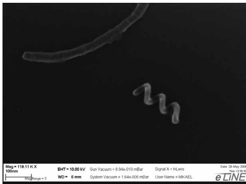
Figure 1. A SEM image of a coiled multiwalled nanotube deposited on a substrate.
