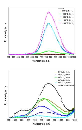
**Fig.1.** Photoluminescence spectra of Si reach  $SiO_2$  layer for different annealing temperatures and annealing time
