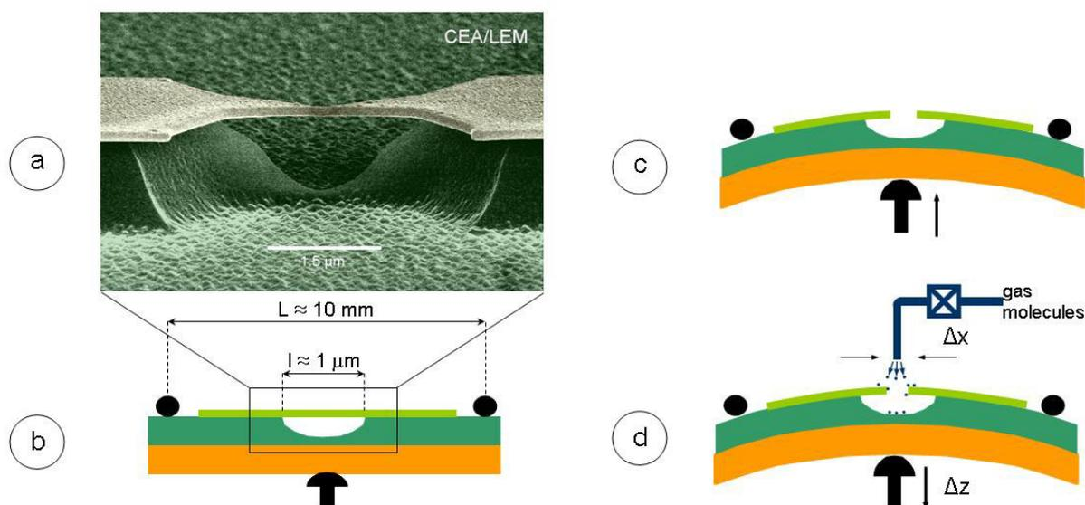
(a) SEM colorized picture. A metallic bridge with dimensions  $\sim 100$  nm is fabricated on an insulating elastic substrate, using conventional e-beam technique. (b) & (c) Using a bending mechanism consisting of 2 side counter-supports and a centred pushing rod, the bridge is elongated until it breaks. (d) The distance between the resulting electrodes is controlled at atomic scale, allowing to connect a single molecule.
