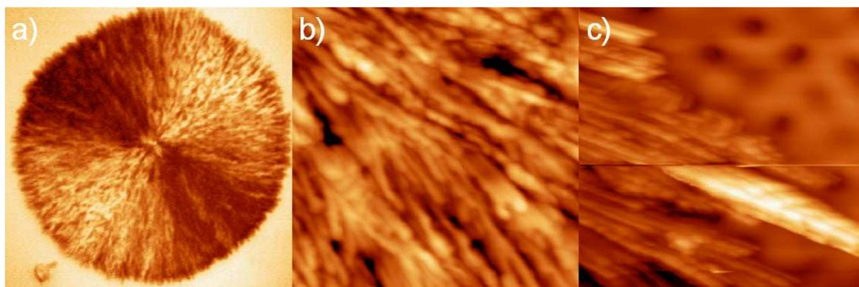
Fig 1. Morphology of rubrene thin films growth on  $\text{SiO}_2$ . a) optical micrographs of rubrene islands. b) AFM image of rubrene crystalline dendrites ( $3\mu\text{m}\times 3\mu\text{m}$ ) c) edge of a polycrystalline island on the amorphous template layer ( $5\mu\text{m}\times 5\mu\text{m}$ ).
