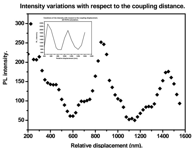
Figure 1 :Extracted intensity variations with respect to the air gap.
