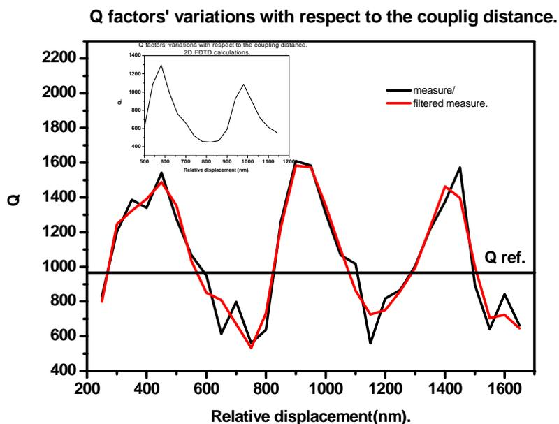
Figure 2 :Quality factor oscillations with respect to the air gap.
