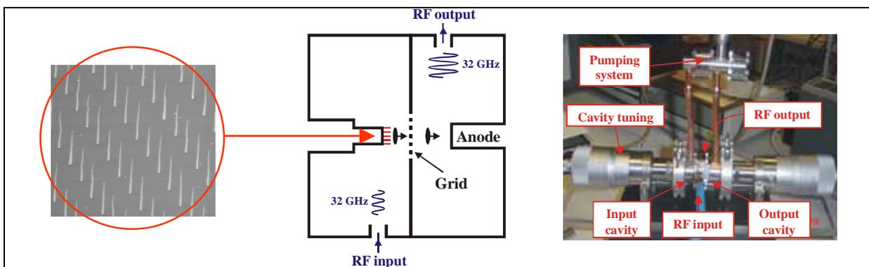
Fig. 3: Array of 2500 CNs (10 μm pitch) integrated in a 32 GHz microtriode. First experiments will be presented
