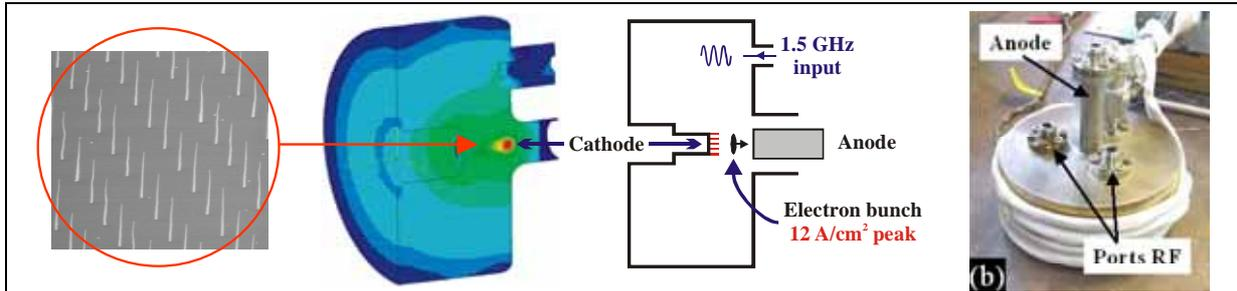
Fig. 2: Array of 2500 CNs (10 μm pitch) integrated in a 1.5 GHz diode. The peak current density is 12 A/cm<sup>2</sup>. K. Teo, E. Minoux et al., *Nature* 437, 968 (2005)
