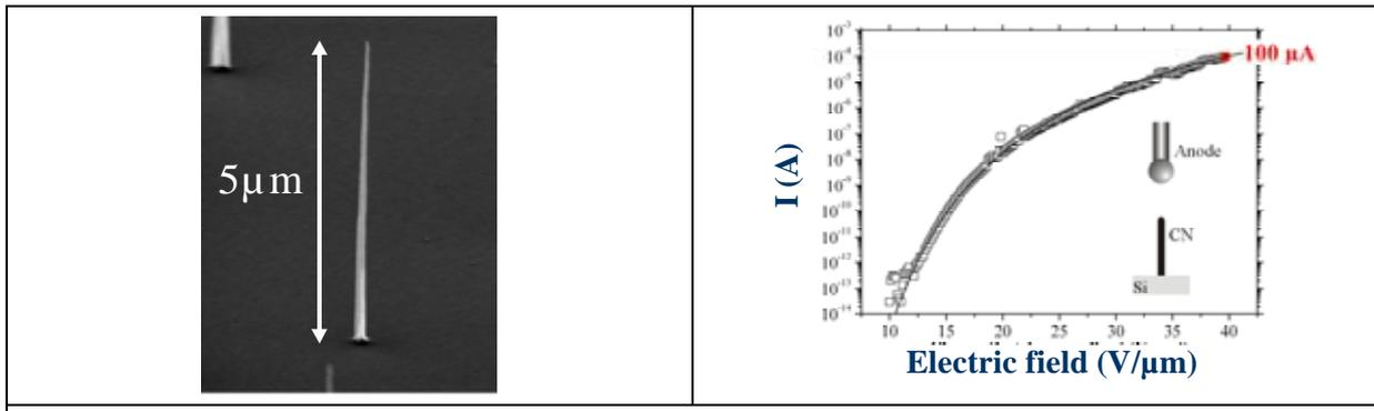
Fig. 1: SEM picture (left) and field emission properties (right) of a 5 μm height and 50 nm diameter CN. E. Minoux et al., *Nano letters* 5, 2135 (2005).
