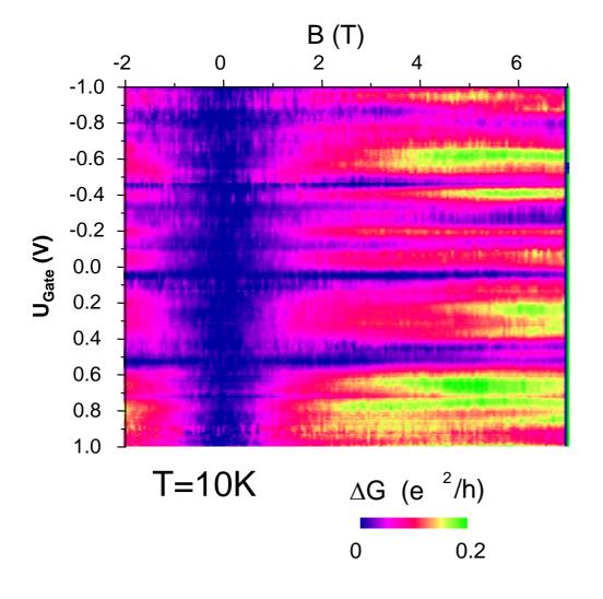
Magneto-conductance of a multiwall carbon nanotube for different gate voltages. The horizontal blue lines correspond to the onset of new conduction subbands.
