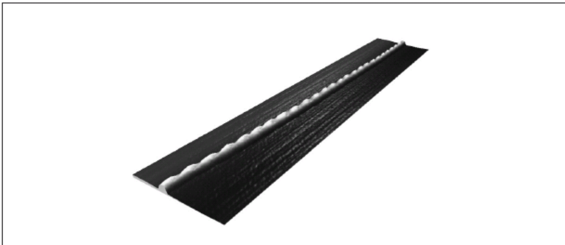
AFM image of an insulin fibril with diameter ~6nm
