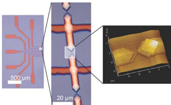
**Figure 2.** Fabrication method for gap (or point contact) structures. All elements shown are fabricated in UHV, using two different masks. (This type of structure is as well used for connecting prefabricated nano-objects.)
