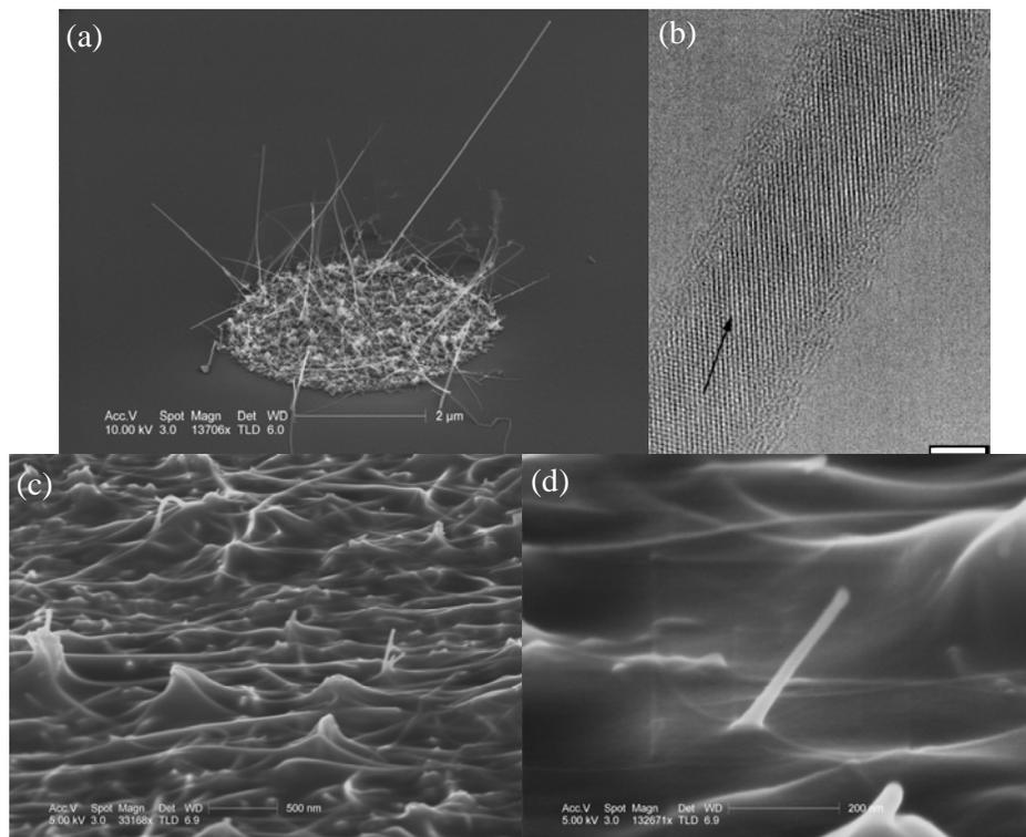
**Fig. 2.** (a) SEM image of SiNWs grown from a catalyst island, (b) HRTEM image of PECVD grown SiNWs (scale bar:  $3\ \text{nm}$ , arrow:  $\langle 111 \rangle$  direction), (c), (d) SEM images of SiNW nanocomposite.
